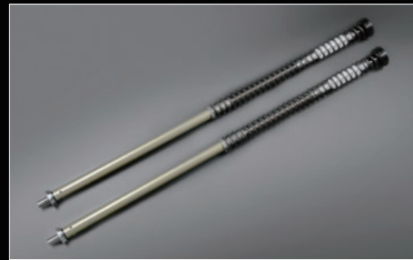
Completely newly designed Technix original cartridge kit example (CRF250L)
