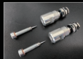
Compression valve side cartridge structure (TRIC)
