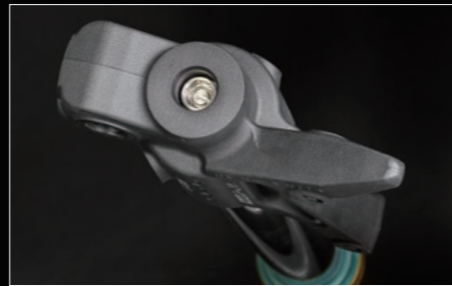
Example of installing a compression adjuster newly installed at the bottom of the fork so that it can be adjusted from the outside (CRF250L)
