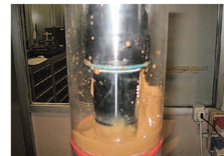
10 hours in mud water to test durability
