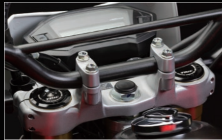
Installation example of the rebound adjuster installed on the top bolt (CRF250L)
