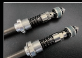
Rebound valve side cartridge structure (TRIC)
